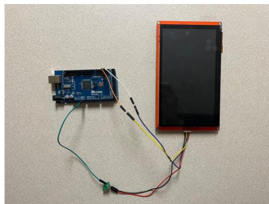
Figure 4: Wiring for the Nextion Display
